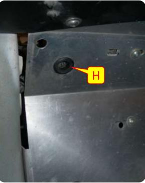
. Install the LED Marker Lights. The Light with the extended leads goes through the front hole (with Gasket) and then through the 1/2" hole in the Inner Fender Well.
